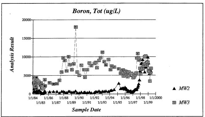
Figure 11. Historical boron concentrations at MW-2 and MW-3.
