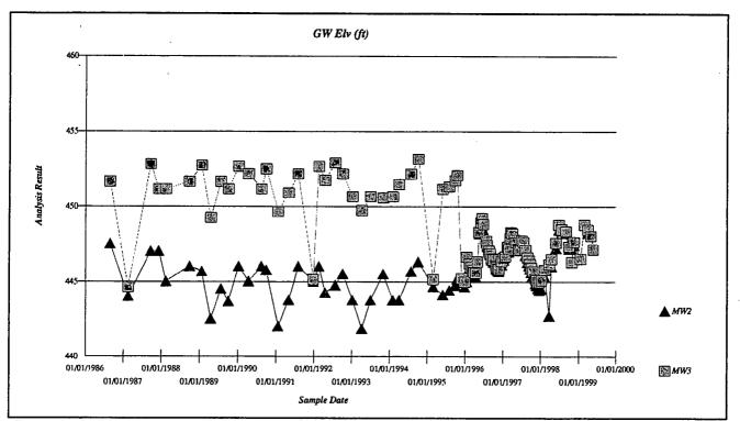
Figure 7. Historical groundwater elevations at MW-2 and MW-3.
